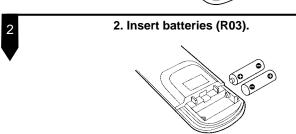
Make sure to match the "+" and "-" of the batteries with the marks inside the battery compartment.
